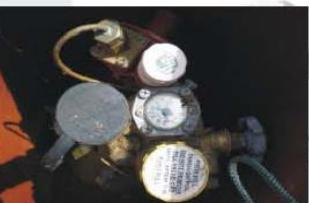
C.) Snap the Remote Ready Sensor into the gauge and re-install on the propane tank. Make sure the propane gauge indicator returns to its original position.
