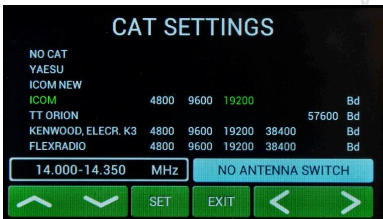
If you choose **YAESU** or **ICOM NEW**, after **SET** pressing you will go to deeper level which allows you to select specific type of TCVR. See the following picture for **ICOM NEW** selection, for example.
