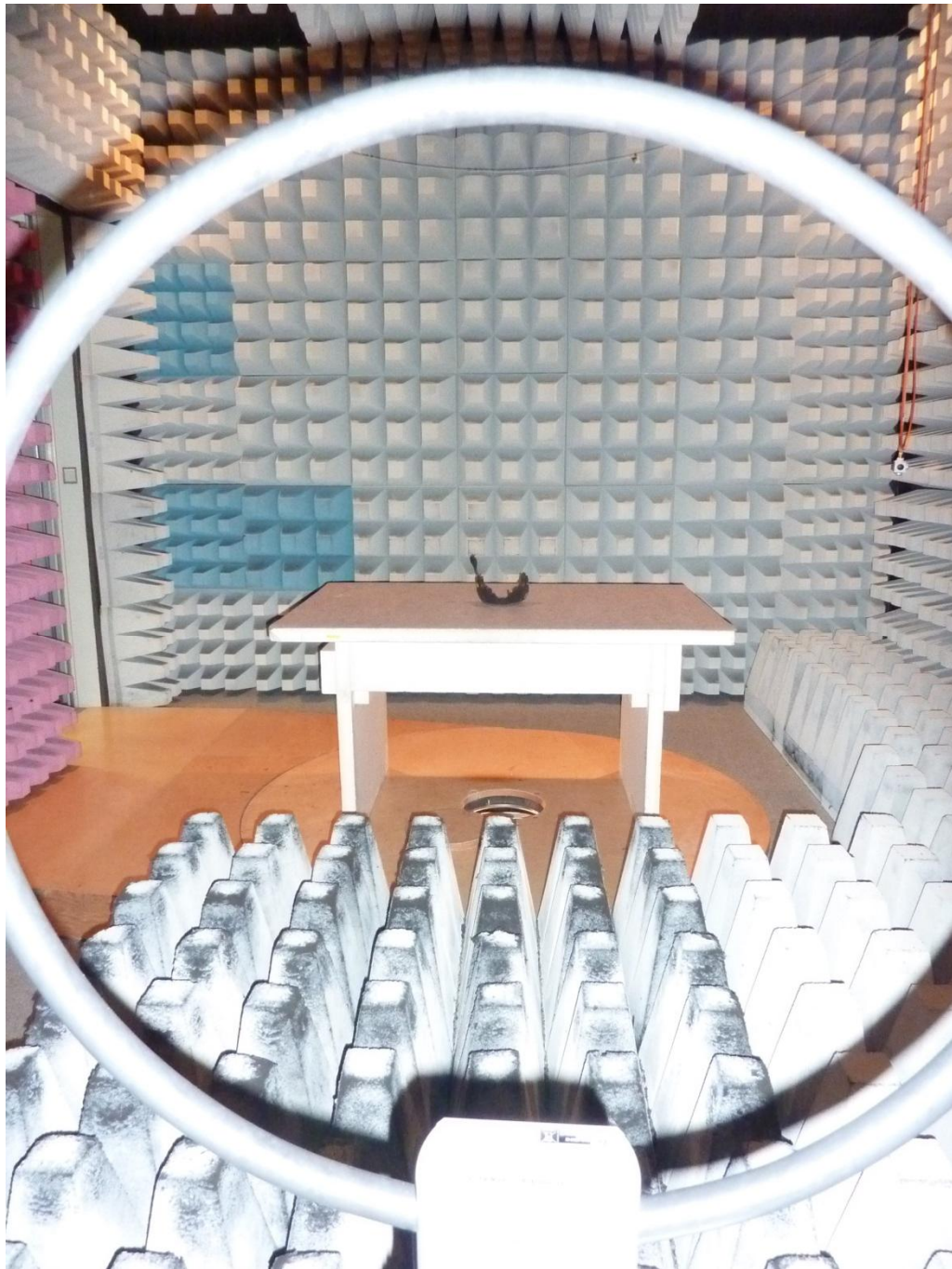
151497_n_i.JPG: FPS COM 7000, test setup fully anechoic chamber
