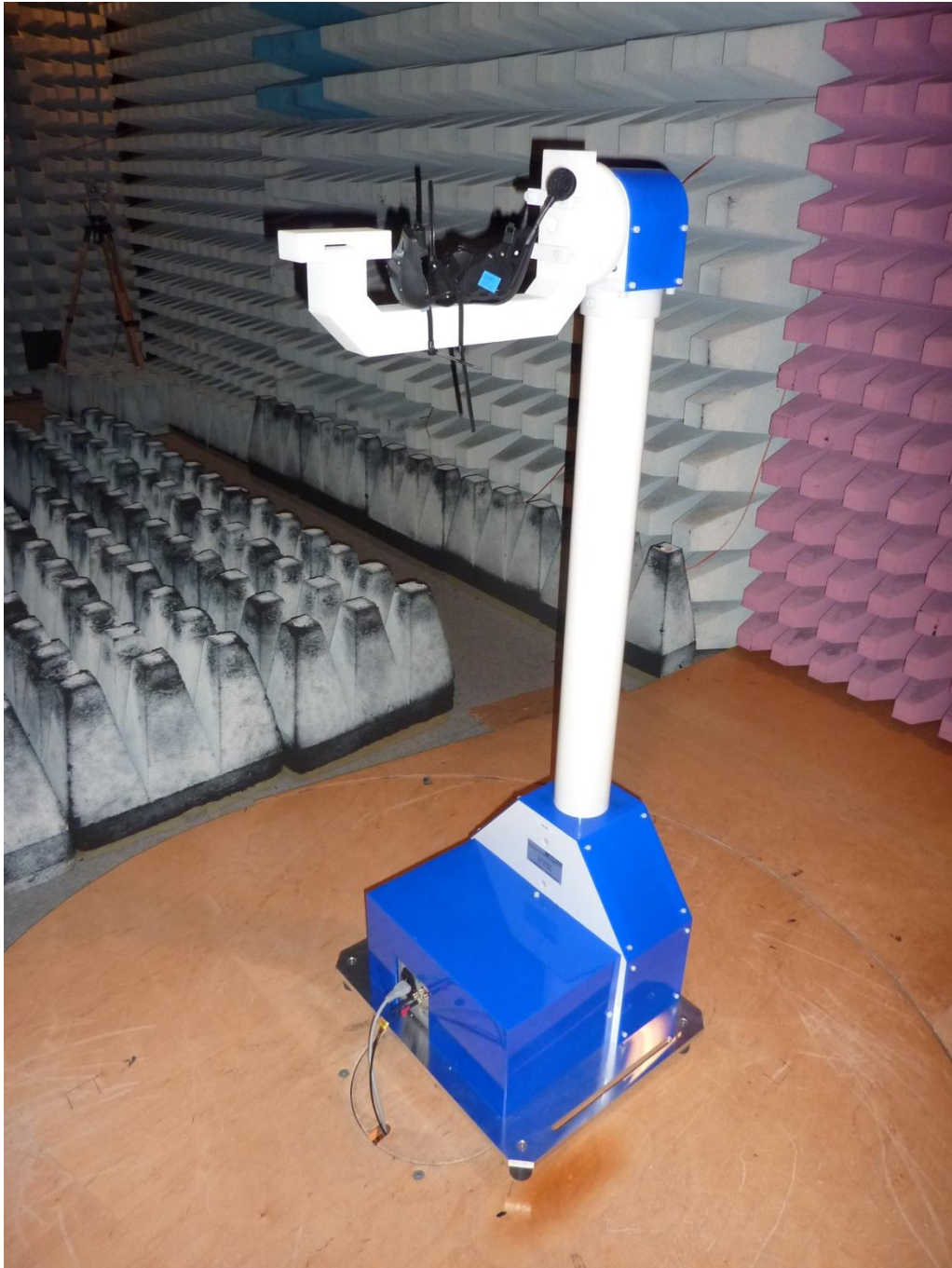
151497_n_f.JPG: FPS COM 7000, test set-up fully anechoic chamber
