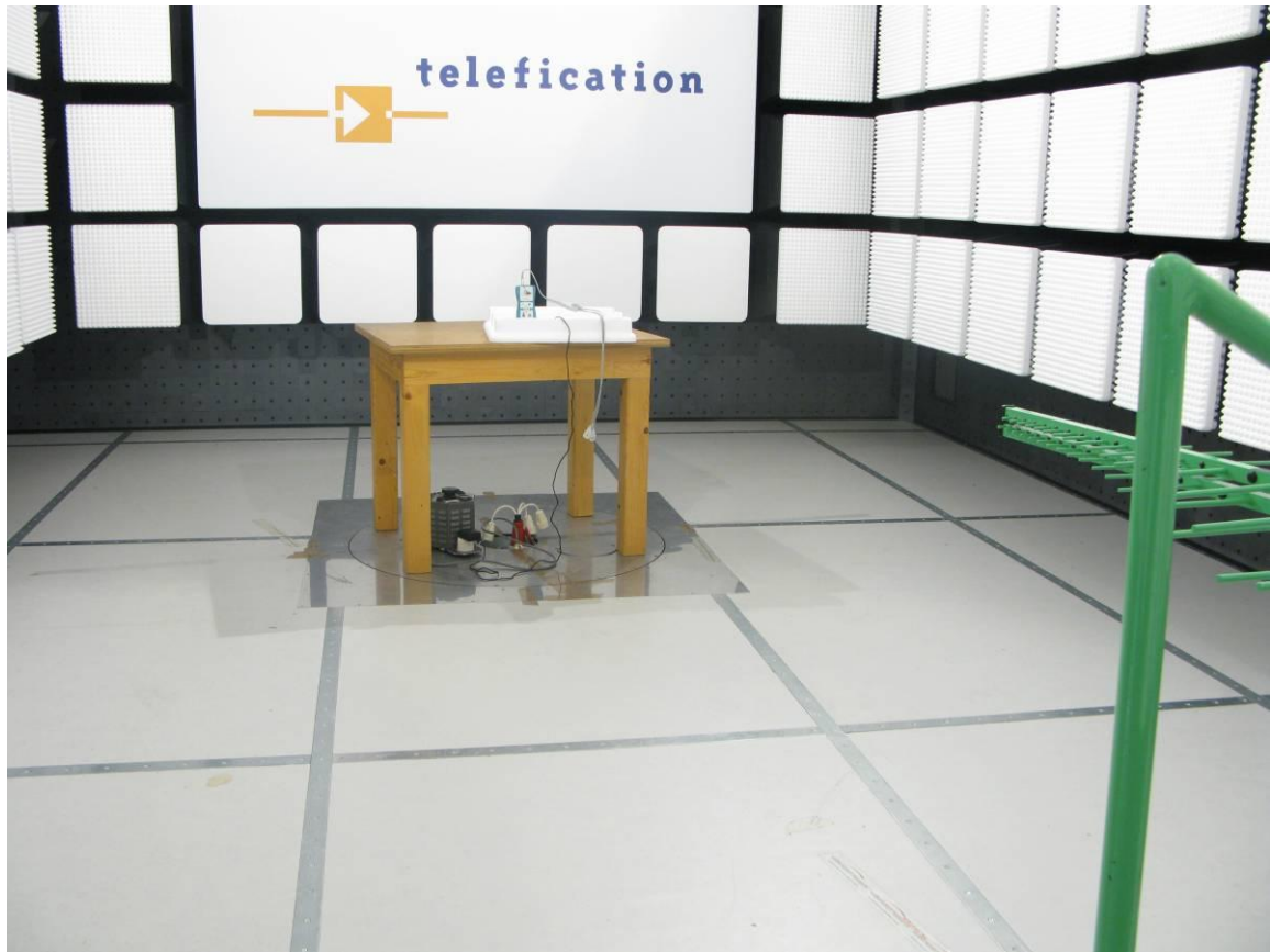
Photograph 4: - Radiated emissions test, photo 4
