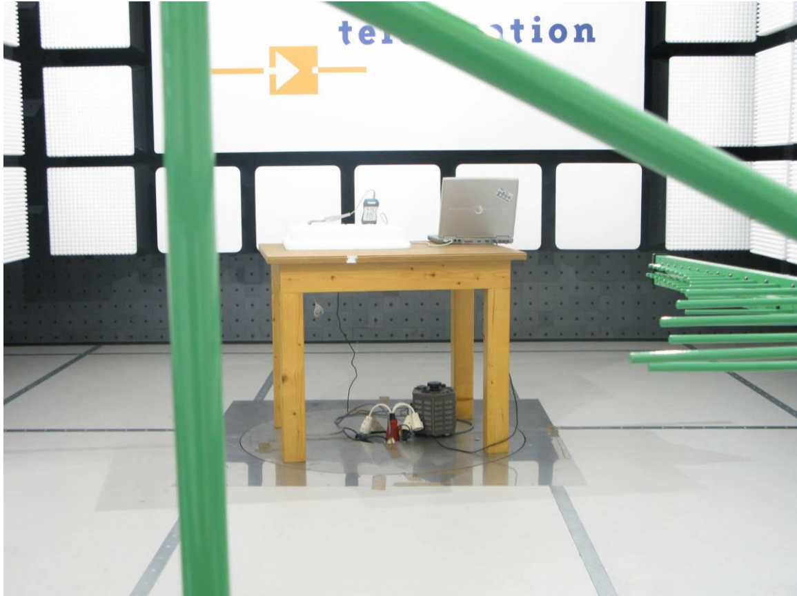
Photograph 2: - Radiated emissions test, photo 2
