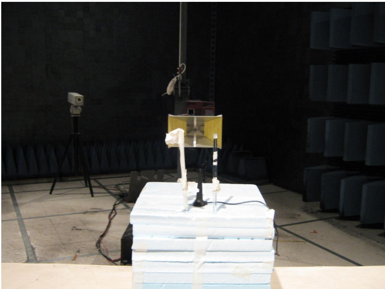
**Radiated Spurious Emissions Test Setup Pictures**
