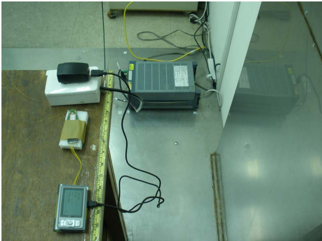
Photo 2: Conducted Emission Test Set-up photo
