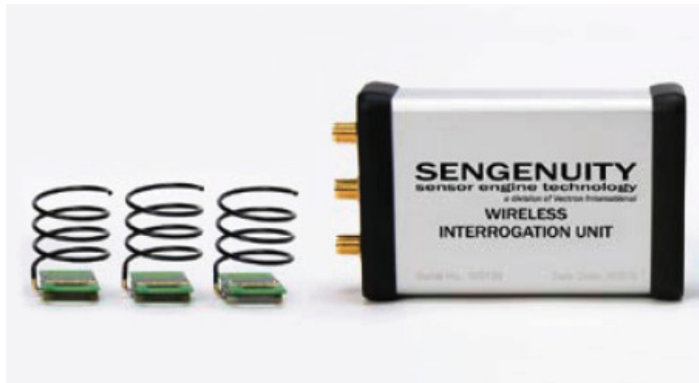
Figure 5. Interrogation unit (reader) and three typical SAW temperature sensor modules. The sensor elements are 3.8\text{mm} \times 3.8\text{mm} ceramic-packaged resonators embedded in the PCB package. The coil antenna shown has been designed for operation in the vicinity of 433 MHz with a desirable radiation pattern.
