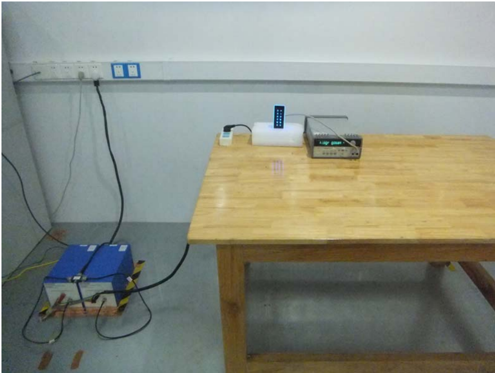
Conducted Emissions Setup Front View
