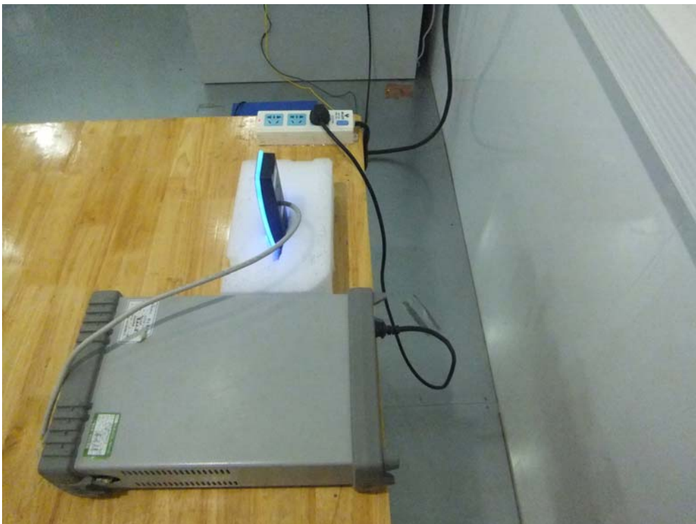
Conducted Emissions Setup Side View
