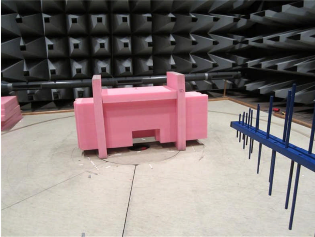
Photo 4.3.1 Test setup regarding measurement of radiated emission.
