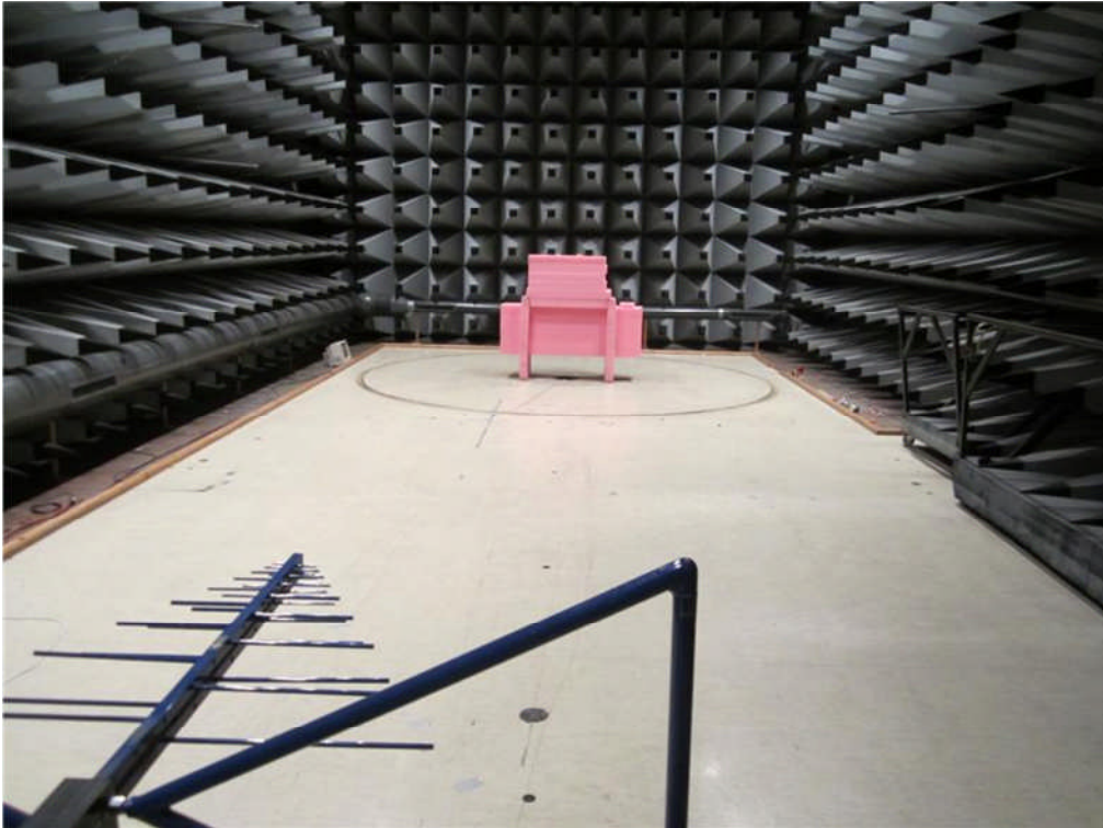
Photo 4.9.1 Test setup regarding measurement of radiated emission, Rx, IC below 1 GHz.
