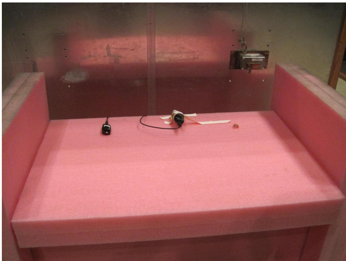
Photo 4.6.1 Test setup regarding measurement of radio frequency voltage on mains.
