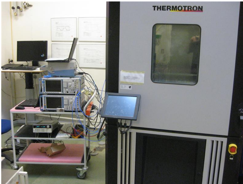
Photo 4.19.1 Test setup regarding measurement of 20 dB bandwidth.
