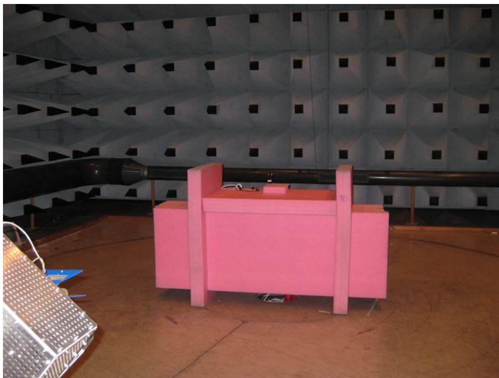
Photo 4.11.1 Test setup regarding measurement of radiated emission above 1 GHz.
