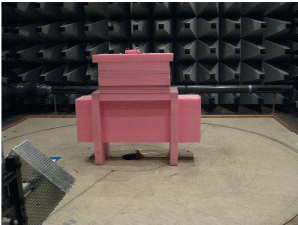
Photo 4.29.1 Test setup regarding measurement of radiated emission above 1 GHz.
