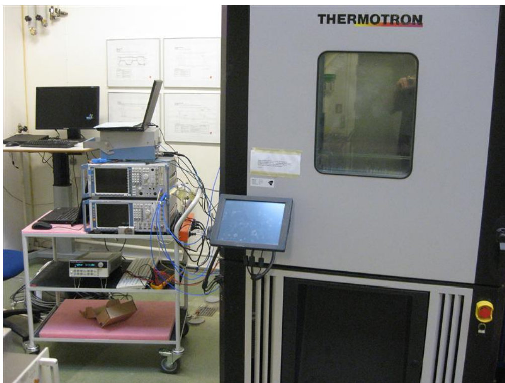
Photo 4.27.1 Test setup regarding measurement of occupied bandwidth, IC.
