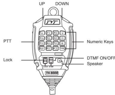
You can operate the transceiver by keypad or input desired frequency or channel through the microphone (Note: In professional transceiver mode, other keys are invalid except PTT, [ **UP** / **DOWN** ], **ON/CALL** and **SET DIAL** ).
