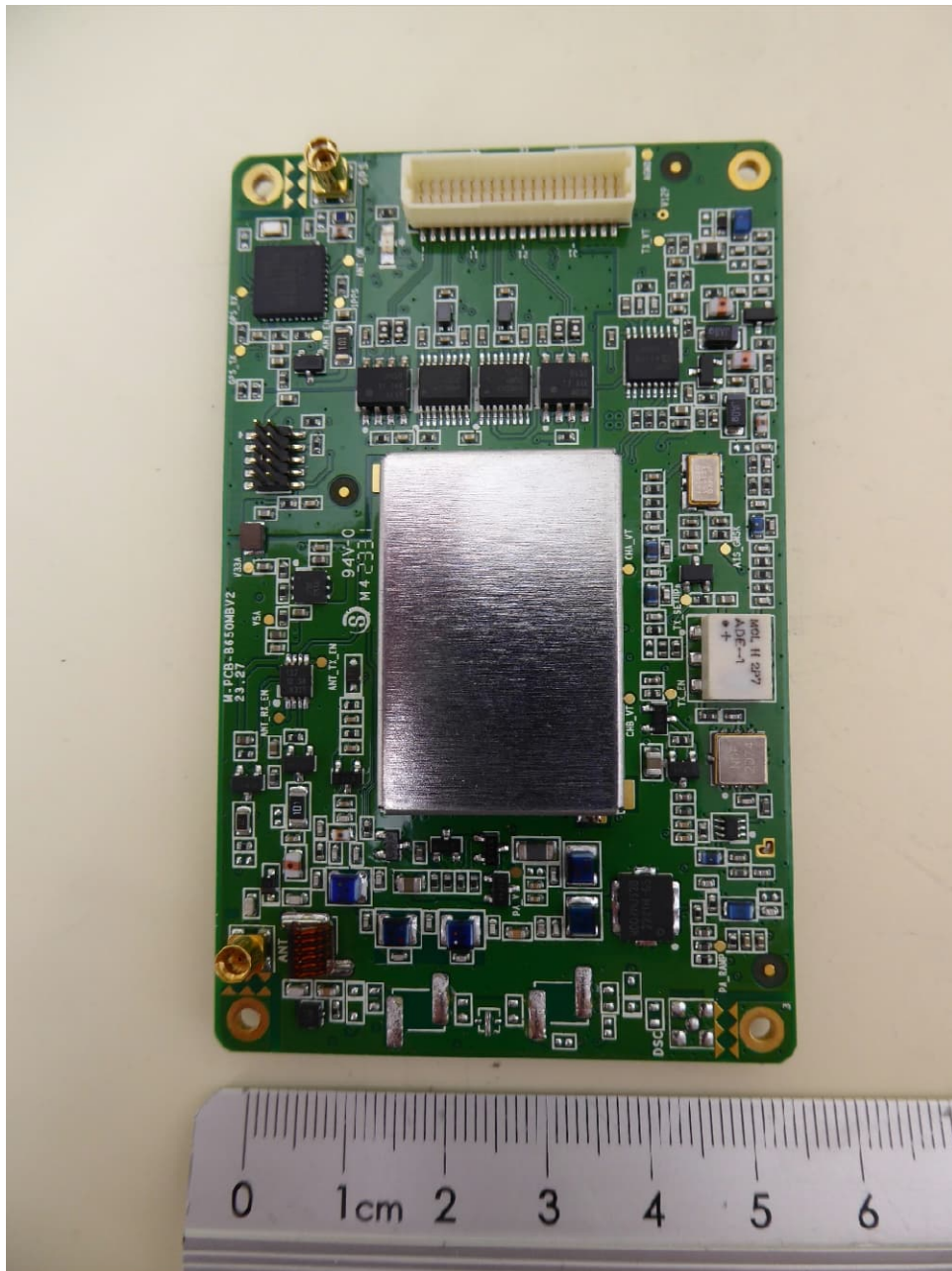
B620 / B620W, main PCB, top view
