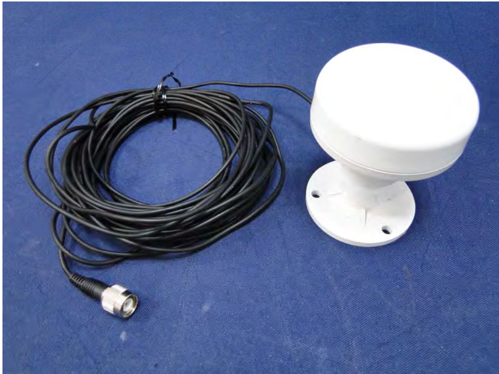
(8) EUT Photo _ GPS antenna with 10m Cable
