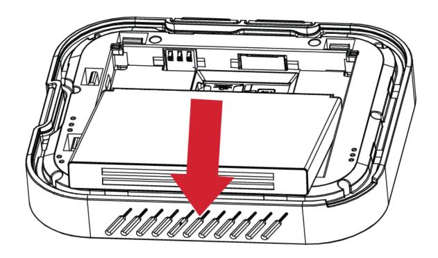
Position the battery in line with the hotspot's gold contacts and slide it gently into place.
