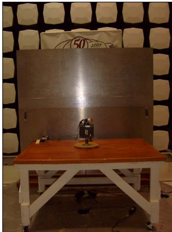
Photograph 8. Conducted Emissions, Test Setup, M5 Radio
