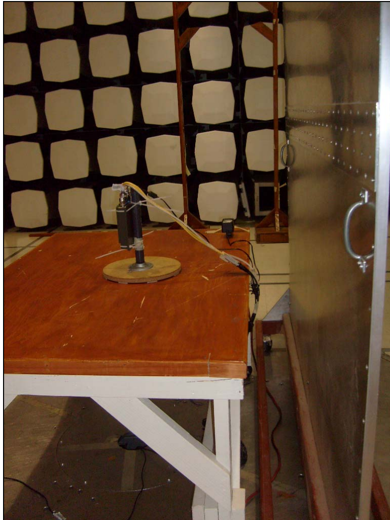
Photograph 9. Conducted Emissions, Test Setup, Side View, M5 Radio
