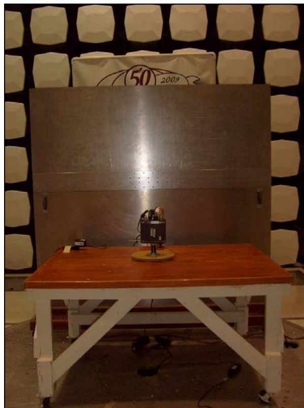
Photograph 3. Conducted Emissions, Test Setup, M25 Radio
