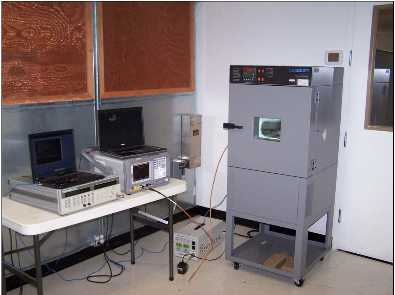
Photograph 11. Frequency Stability, Test Setup, M5 Radio
