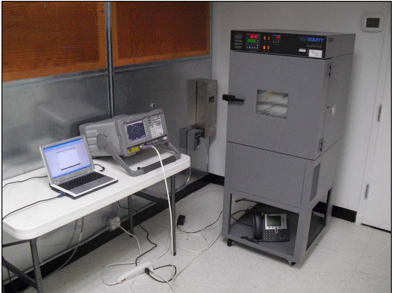
Photograph 6. Frequency Stability, Test Setup, M25 Radio
