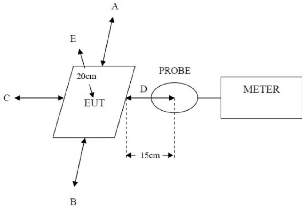
Note: Measurements should be made from all sides and the top of EUT, with the 15cm measured from the center of the probe(s) to the edge of the device and the 20cm measured from the center of the probe(s) to the top of the device. Position A is the front of the EUT, position B is the rear of the EUT, position C is the left of the EUT, position D is the right of the EUT, position E is the top of the EUT.
