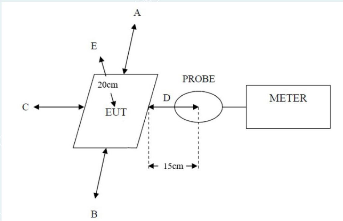
Note: Measurements should be made from all sides and the top of EUT, with the 15cm measured from the center of the probe(s) to the edge of the device and the 20cm measured from the center of the probe(s) to the top of the device. Position A is the front of the EUT, position B is the rear of the EUT, position C is the left of the EUT, position D is the right of the EUT, position E is the top of the EUT.
