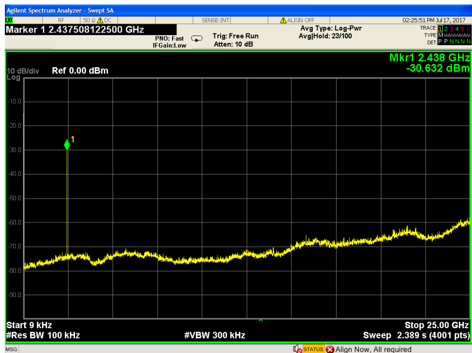
Middle Channel 9 KHz -25GHz Conducted Spurious
