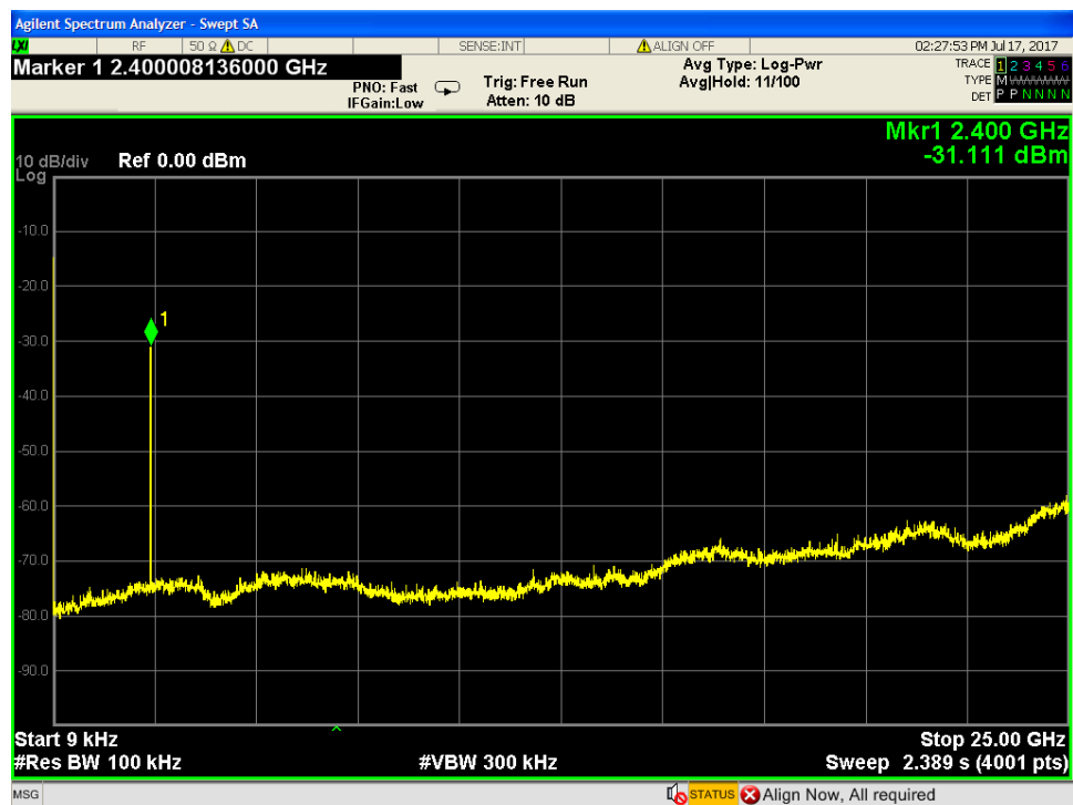
Low Channel 9 KHz -25GHz Conducted Spurious
