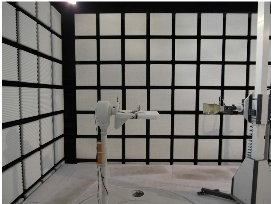
Photo 5: EUT at the anechoic chamber
