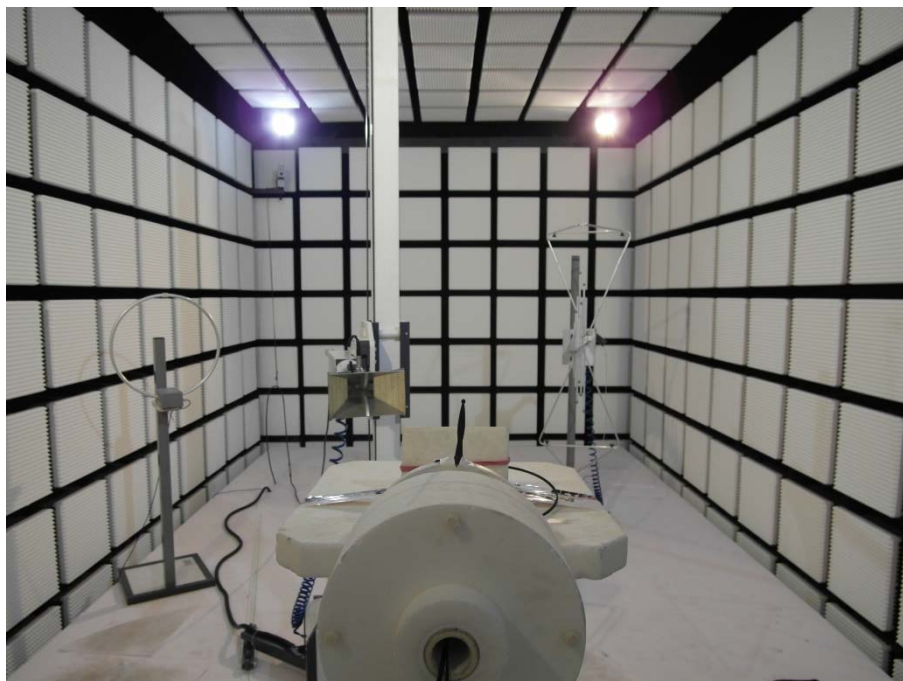
Photo 4: EUT at the anechoic chamber
