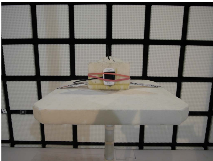
Photo 2: EUT at the anechoic chamber
