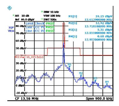
Remark: \*\(^1\) noise floor noise level of the measuring instrument \(^2 4.0 \dB\mu V \@ 10 m \distance \((0.009 - 30 \dMHz)\)
