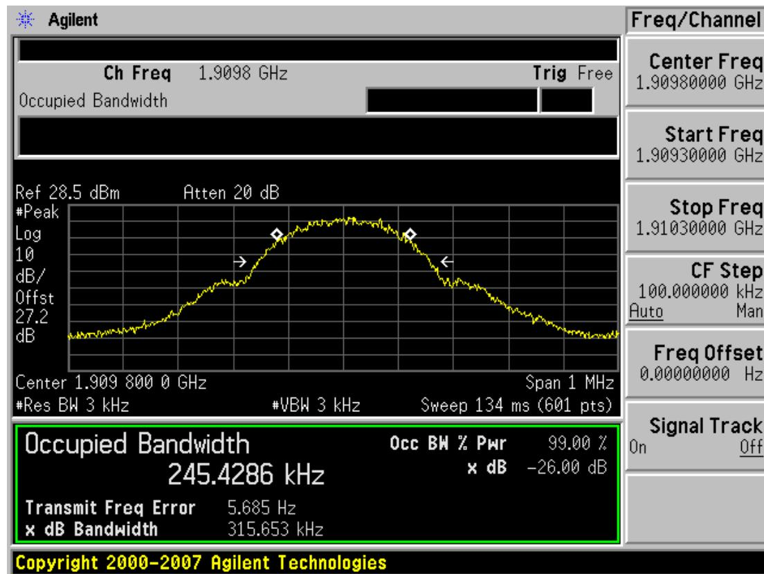
■ GSM1900 EDGE MODE (661 CH.) Occupied Bandwidth
