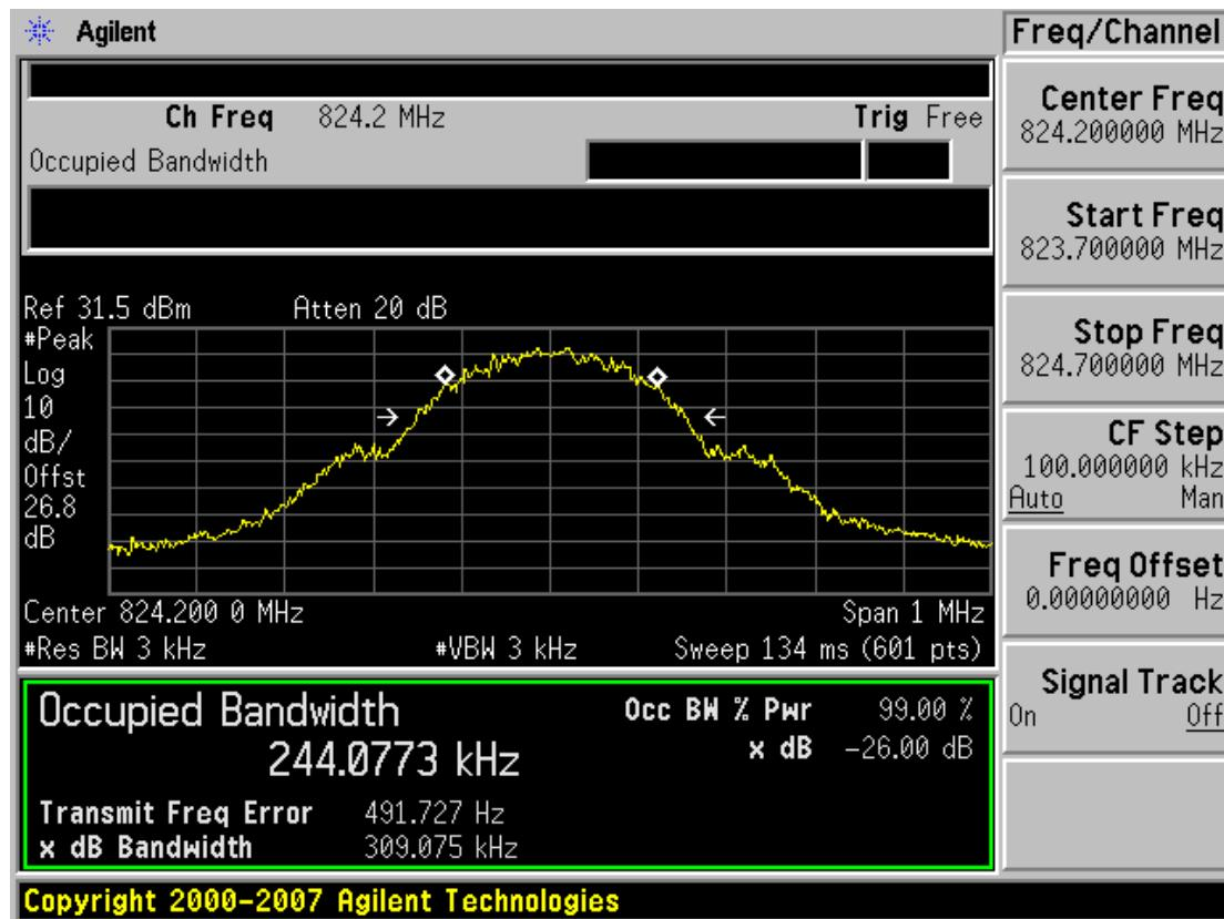
■ GSM850 MODE (190 CH.) Occupied Bandwidth
