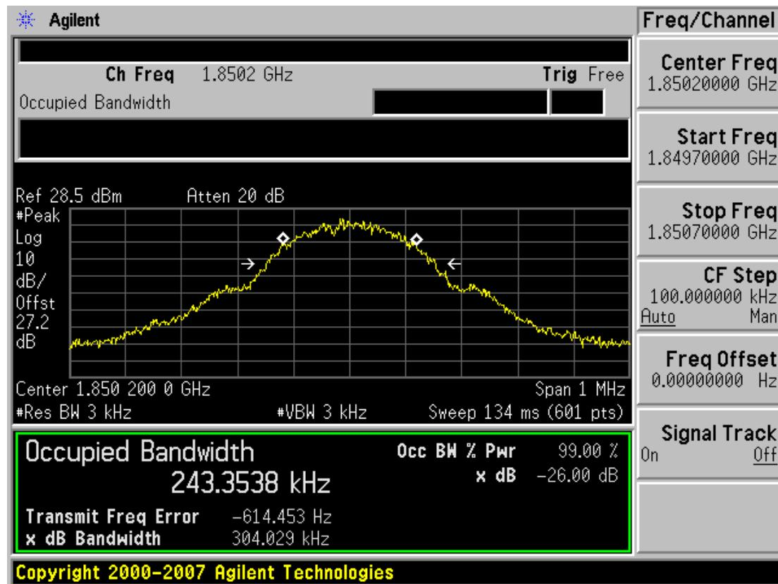
■ GSM1900 MODE (661 CH.) Occupied Bandwidth
