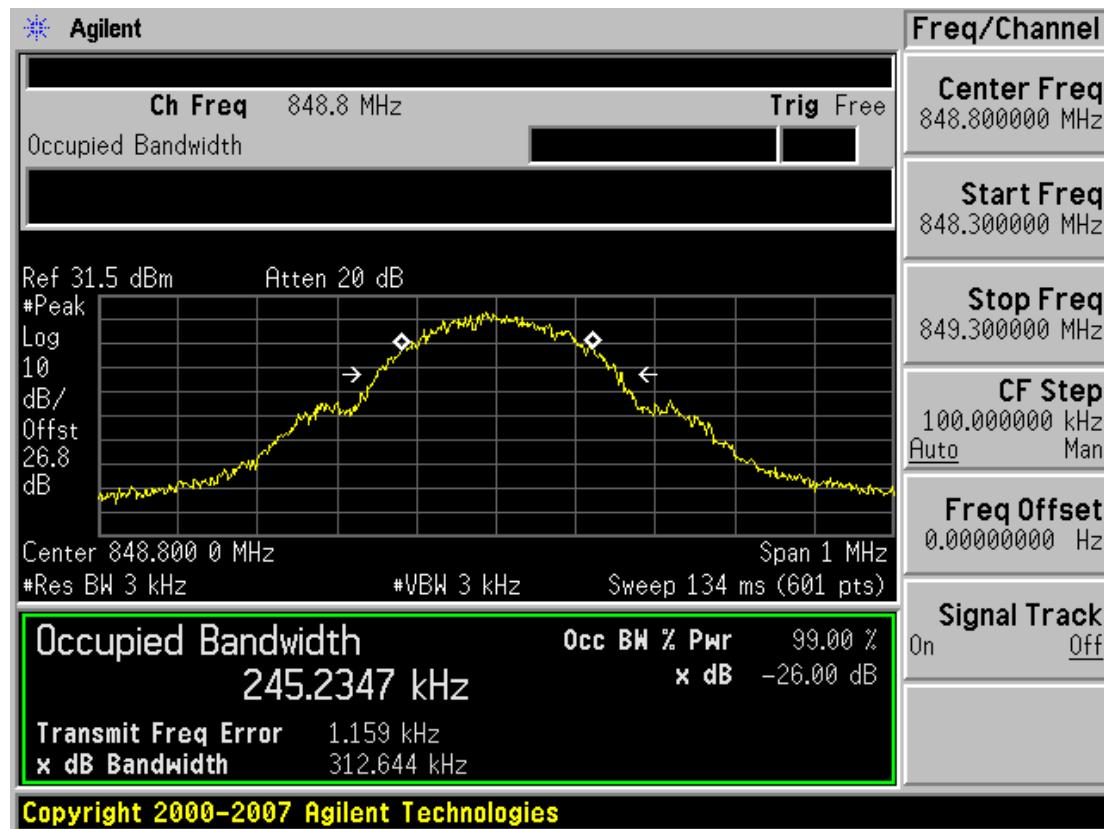
■ GSM850 EDGE MODE (251 CH.) Occupied Bandwidth
