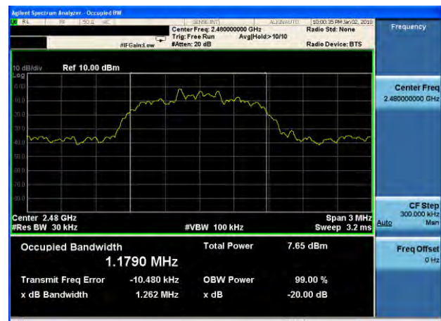
20dB Bandwidth plot on channel 78 (2Mbps)
