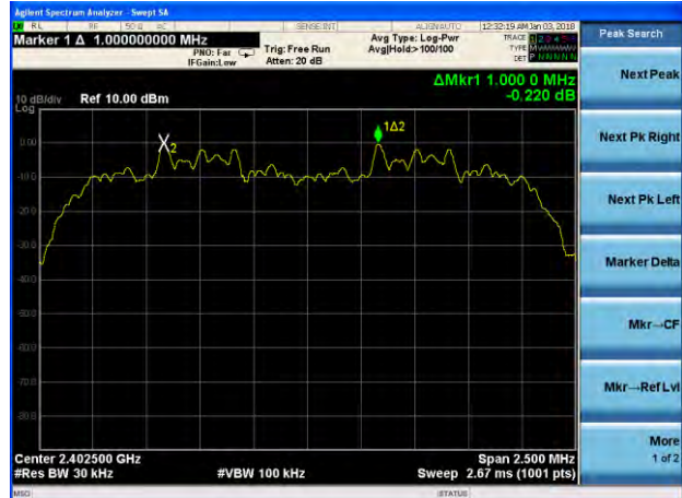
(2Mbps) Channel Separation plot on channel 39-40
