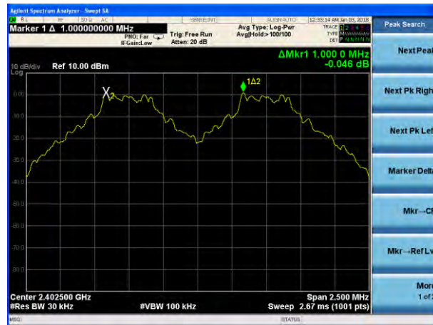
(1Mbps) Channel Separation plot on channel 39-40
