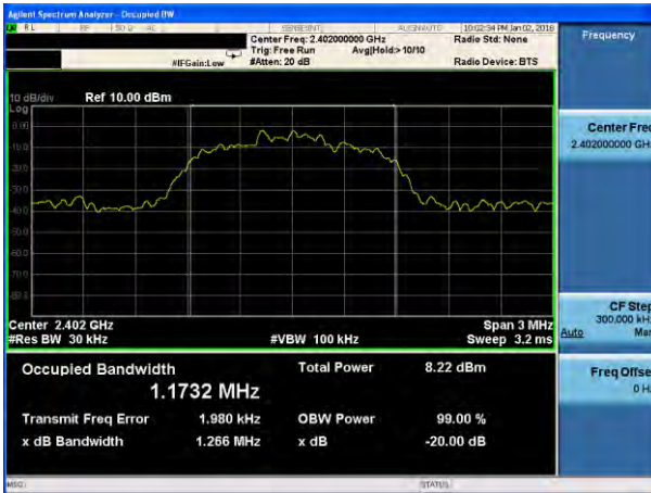
20dB Bandwidth plot on channel 39 (3Mbps)
