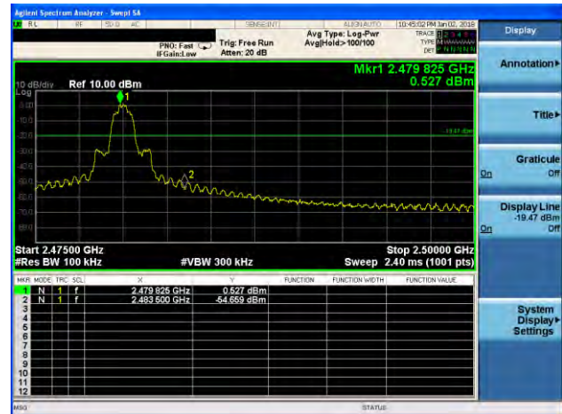
\pi /4-DQPSK: Band Edge-High Channel (Hopping Mode)
