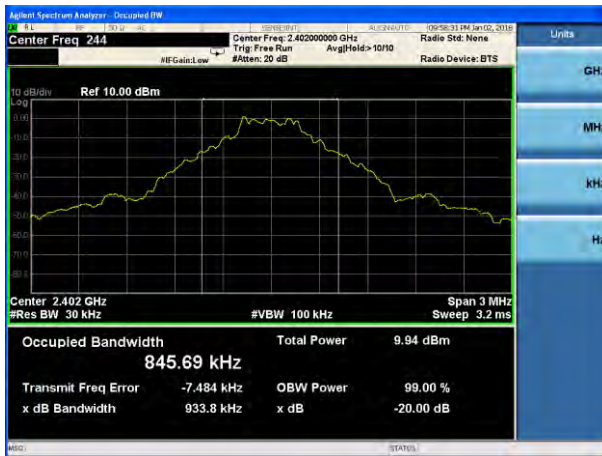
20dB Bandwidth plot on channel 39 (1Mbps)
