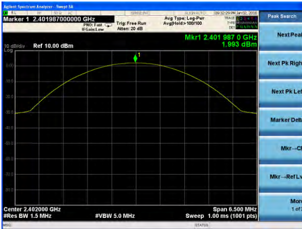
Peak output Power plot on channel 39 (3Mbps)
