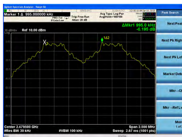
(1Mbps) Channel Separation plot on channel 77-78
