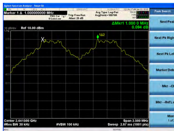
(1Mbps) Channel Separation plot on channel 39-40
