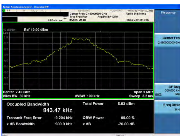
20dB Bandwidth plot on channel 78 (1Mbps)
