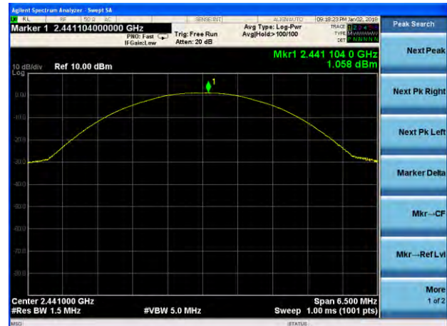
Peak output Power plot on channel 39 (2Mbps)
