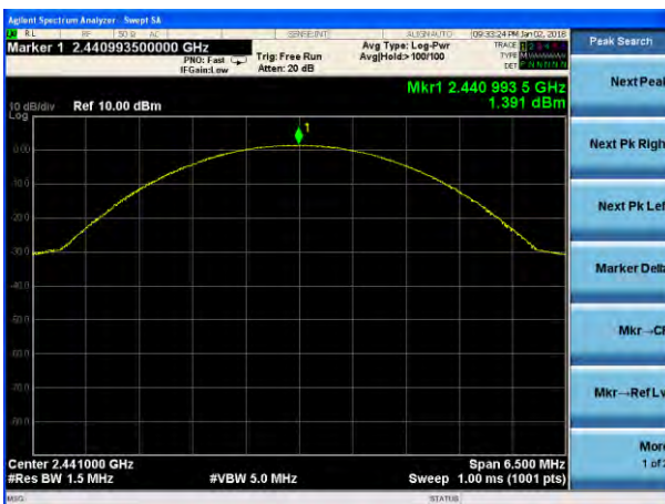
Peak output Power plot on channel 39 (3Mbps)
