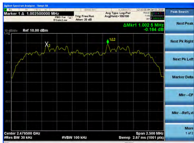
(2Mbps) Channel Separation plot on channel 77-78
