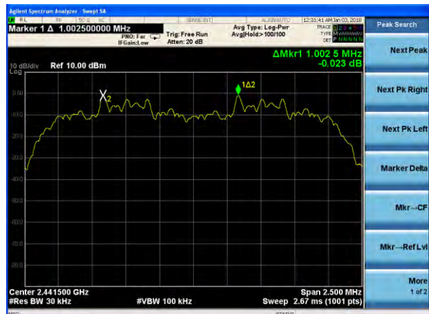
(2Mbps) Channel Separation plot on channel 39-40
