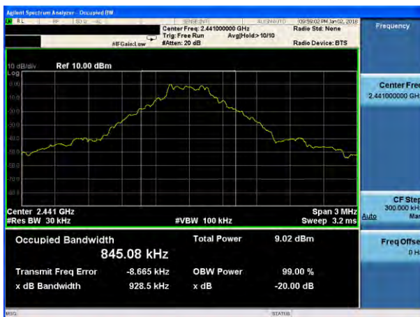
20dB Bandwidth plot on channel 39 (1Mbps)
