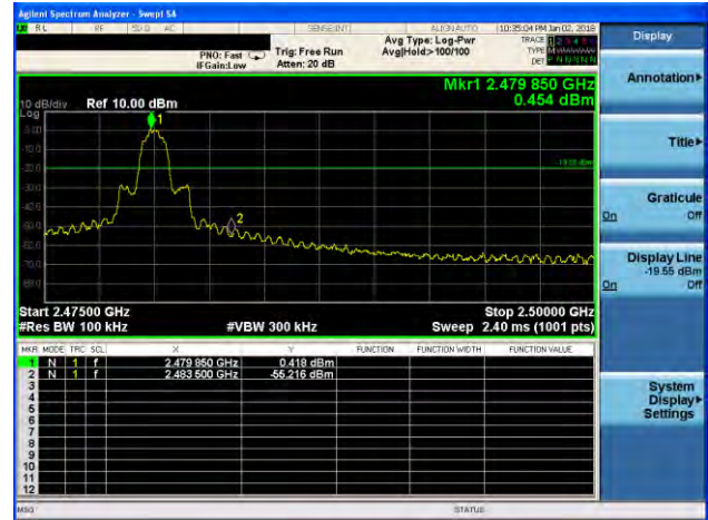
8-DPSK: Band Edge-High Channel
