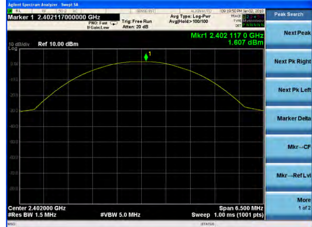
Peak output Power plot on channel 39 (2Mbps)
