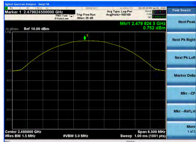
Peak output Power plot on channel 78 (2Mbps)
