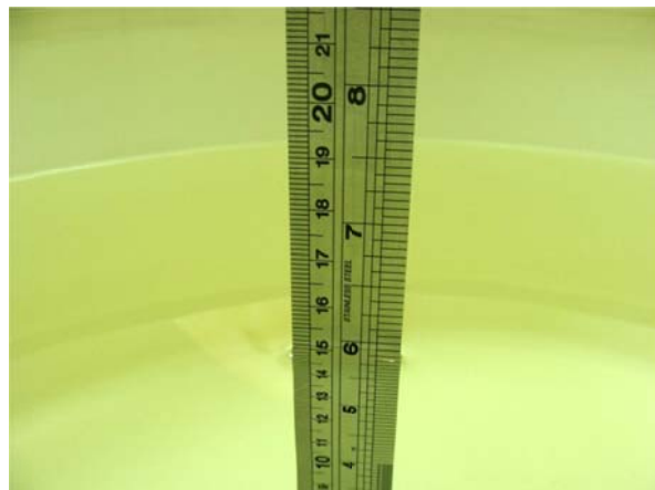
Fig 6.2 Photo of Liquid Height for Body SAR
