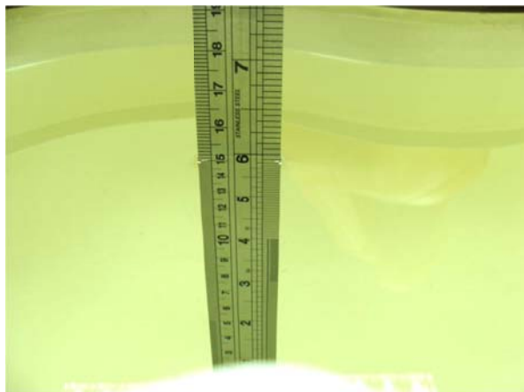
Fig 6.1 Photo of Liquid Height for Head SAR
