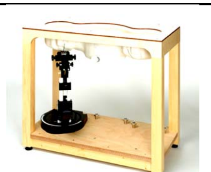
Fig 5.2 Photo of SAM Phantom
