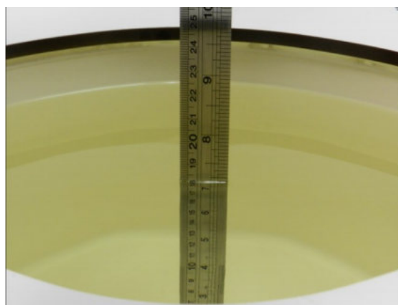
Fig 10.2 Photo of Liquid Height for Body SAR
