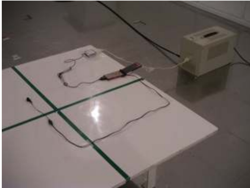
AC Power Line emission
