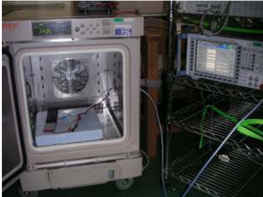
Temperature test (Frequency Stability)
