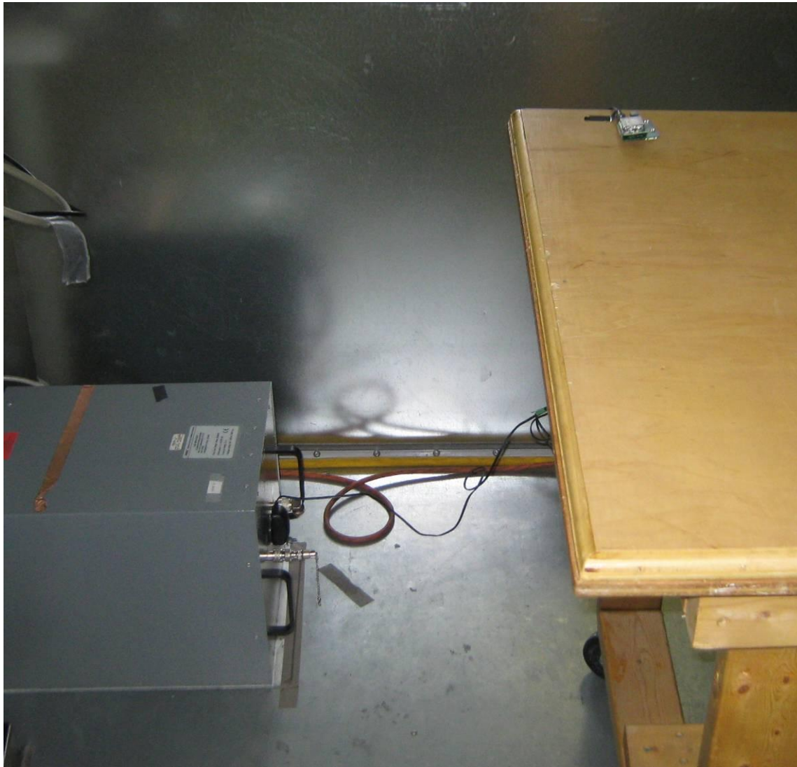
Power Line Conducted Emissions Setup
