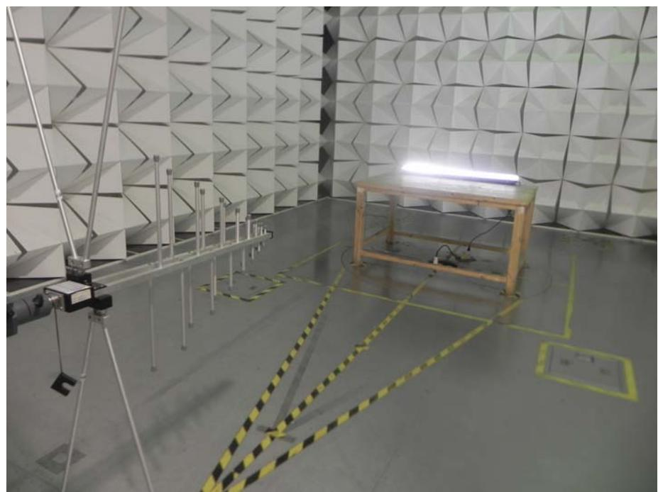
Test frequency above 1GHz at test site 1#
