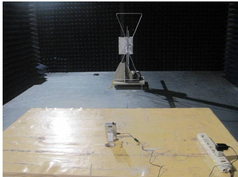
**Radiation Emission Test View For 1GHz-25GHz**
