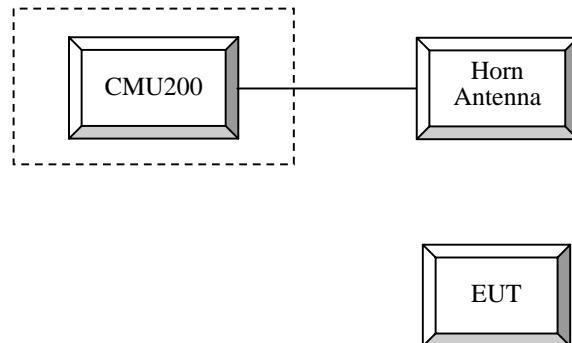
**Block Diagram of Test Setup**
