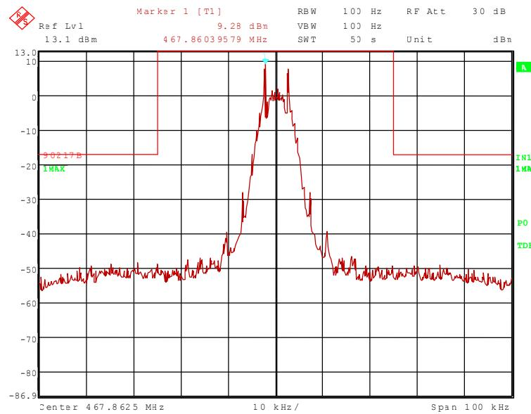
60942\_15.wmf: Spectrum mask, transmitter operates with burst modulation on 467.8625 MHz:
