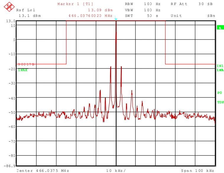
60942\_11.wmf: Spectrum mask, transmitter operates continuous modulation on 466.0375 MHz:
