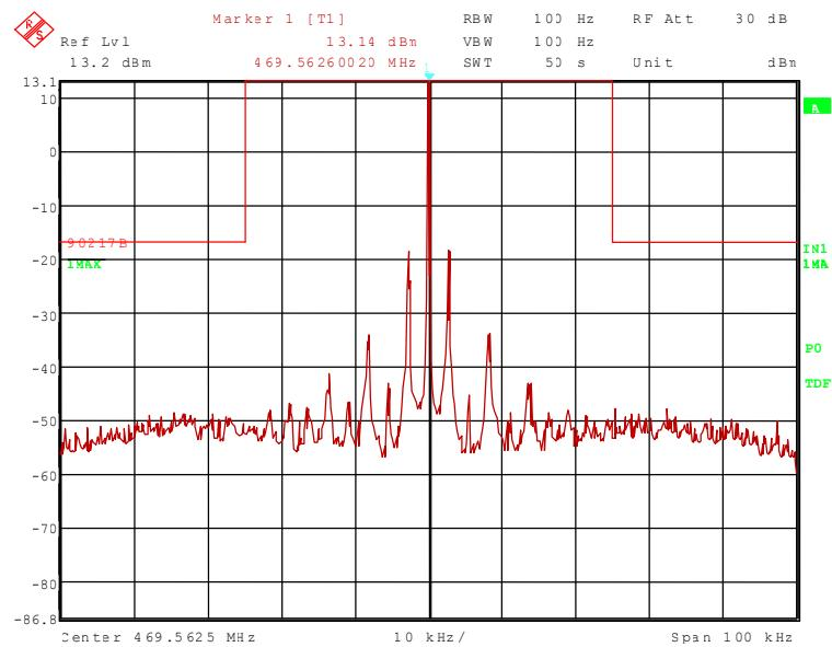
60942\_17.wmf: Spectrum mask, transmitter operates continuous modulation on 469.5625 MHz:
