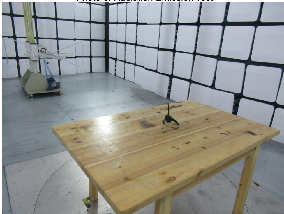
Photo of Radiation Emission Test
