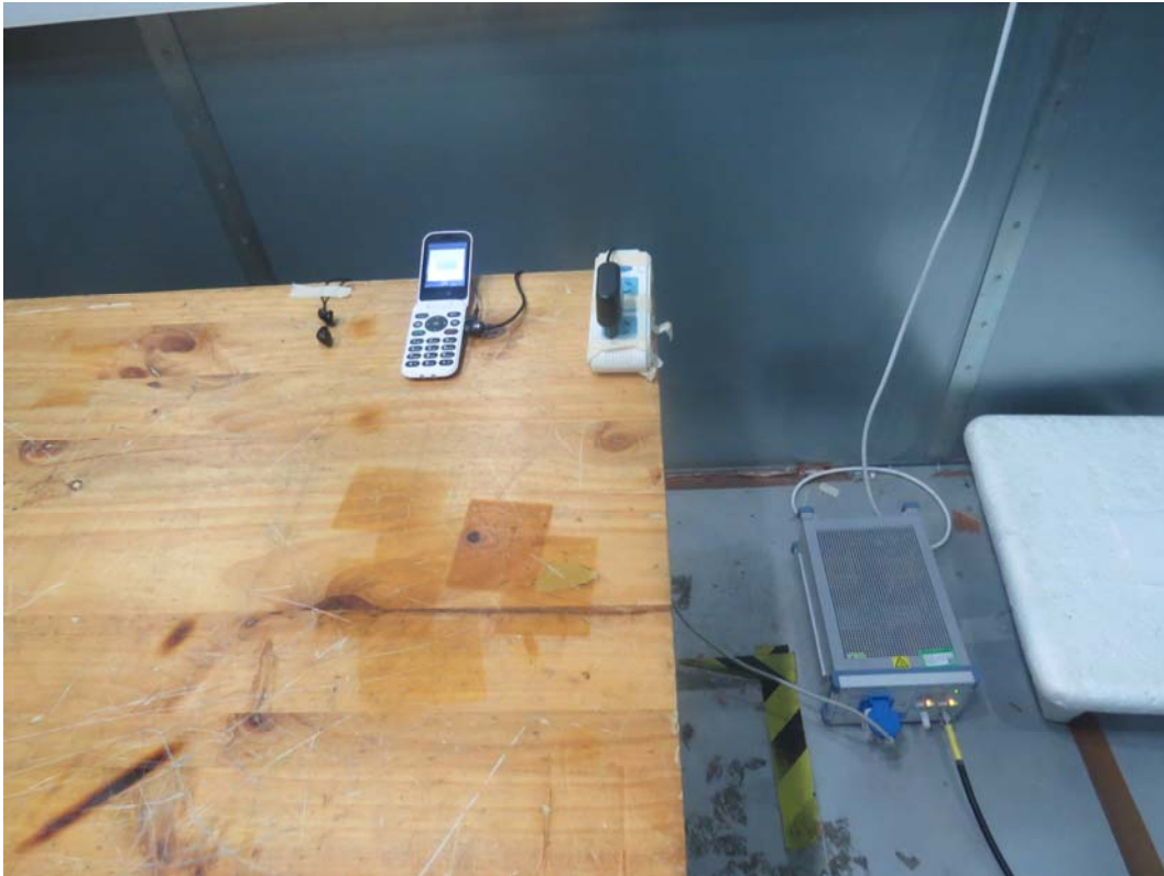
Picture 3 Conducted Emission Test Setup
