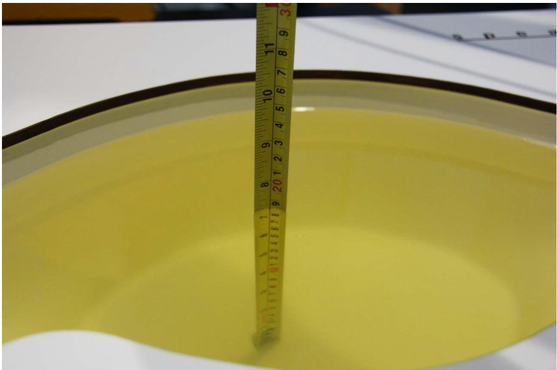
Picture 7-8: Liquid depth in the Flat Phantom(2450MHz)
