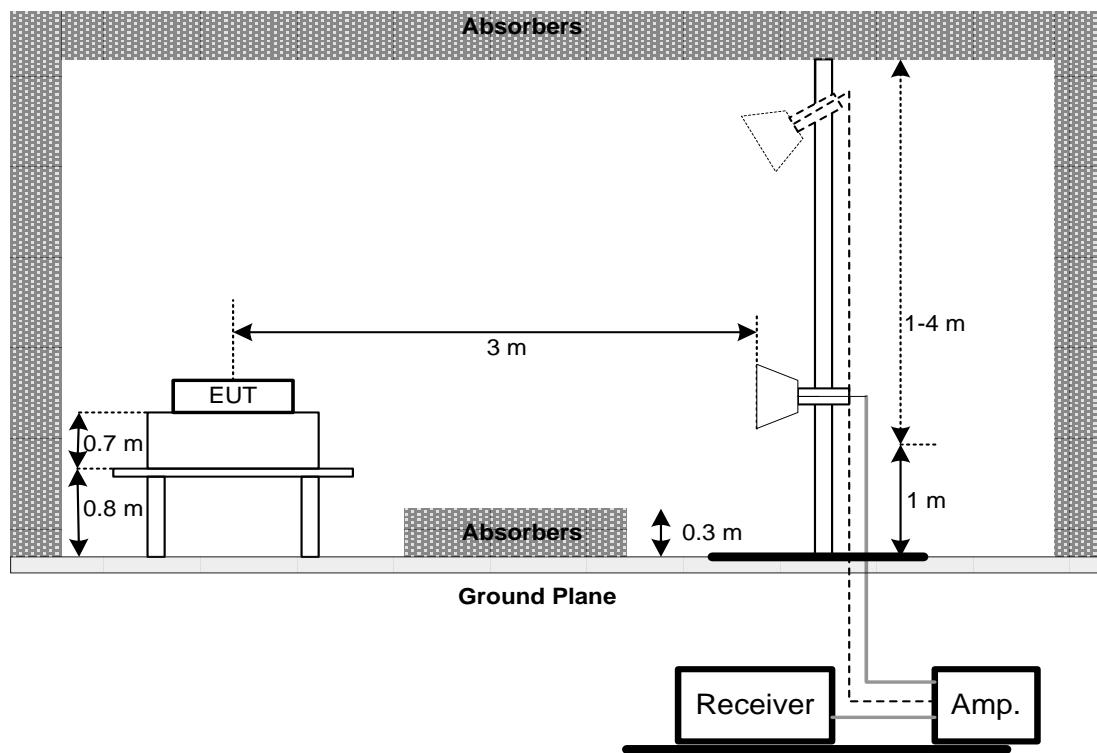
(C) For Radiated Emissions Below 30MHz
