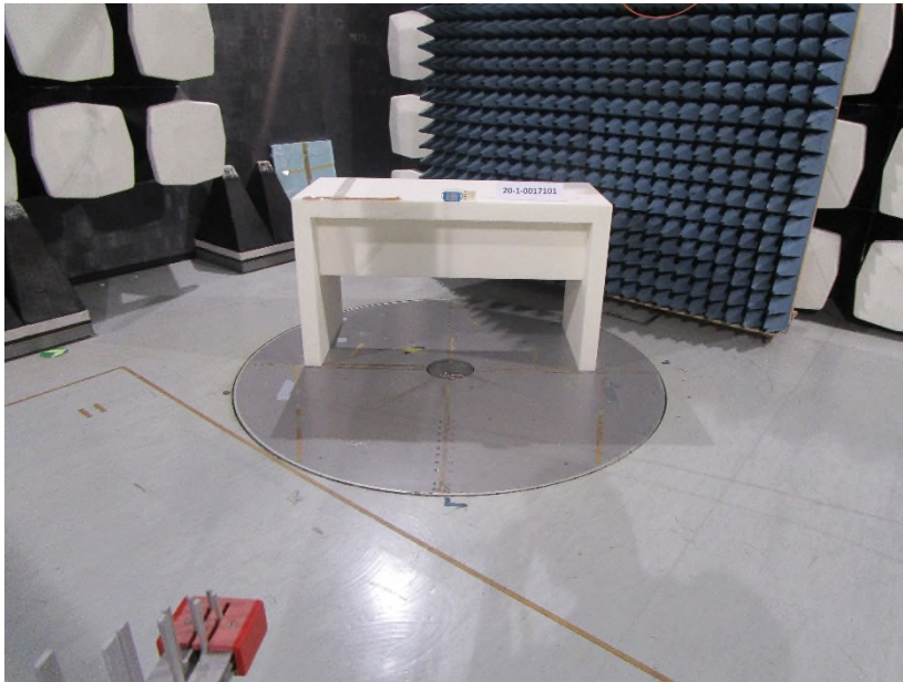
Photograph 1: EUT Test Setup in the anechoic chamber, overview
