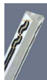
Figure 3.2 Probe Thick-Film Technique
