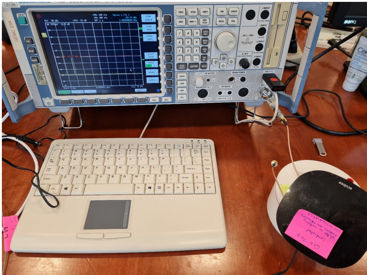
Figure 5 – Antenna Port Conducted Emissions Setup
