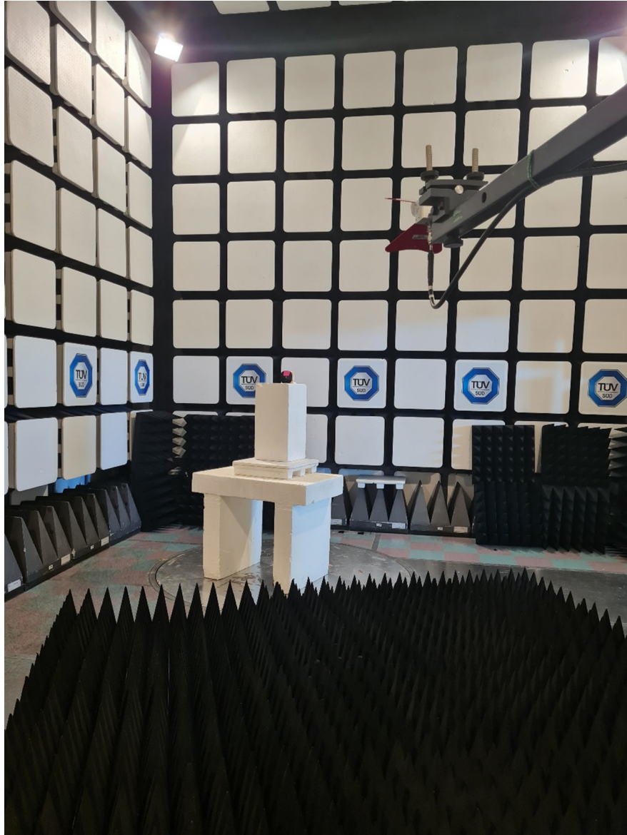
Figure 3 – Radiated Emissions Setup > 1GHz
