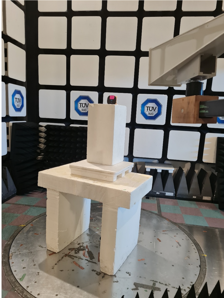
Figure 4 – Radiated Emissions Setup > 1GHz
