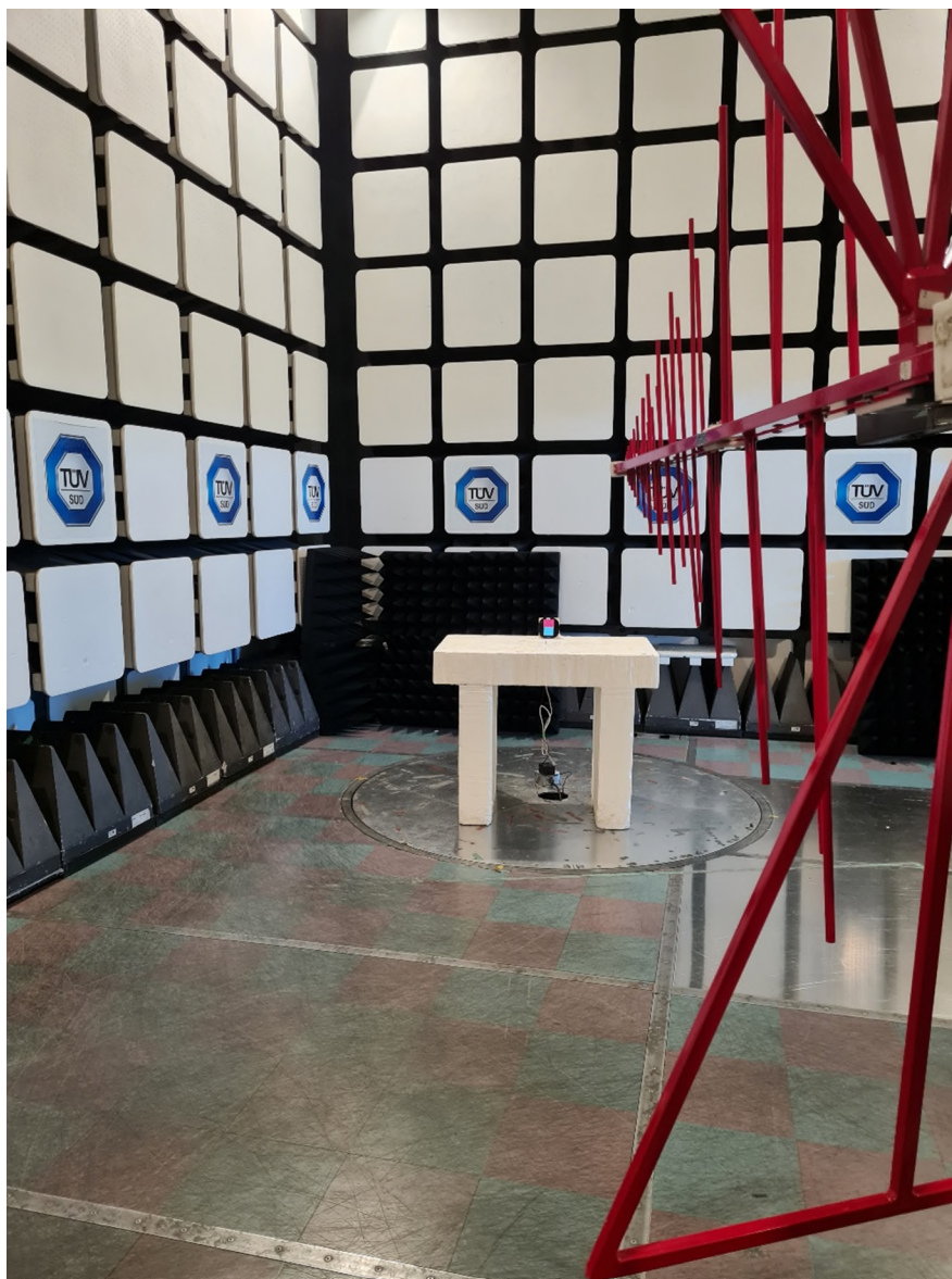
Figure 2 – Radiated Emissions Setup 30MHz – 1GHz
