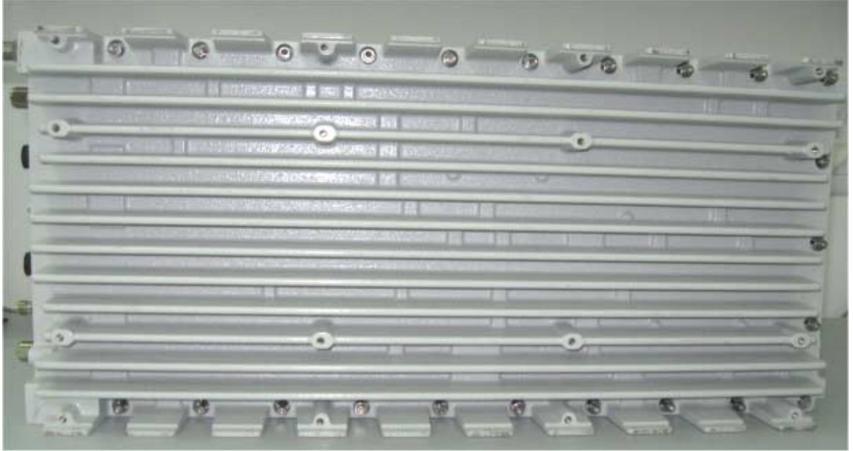
Photograph No.3 Base station WiN7037-2 rear side view
