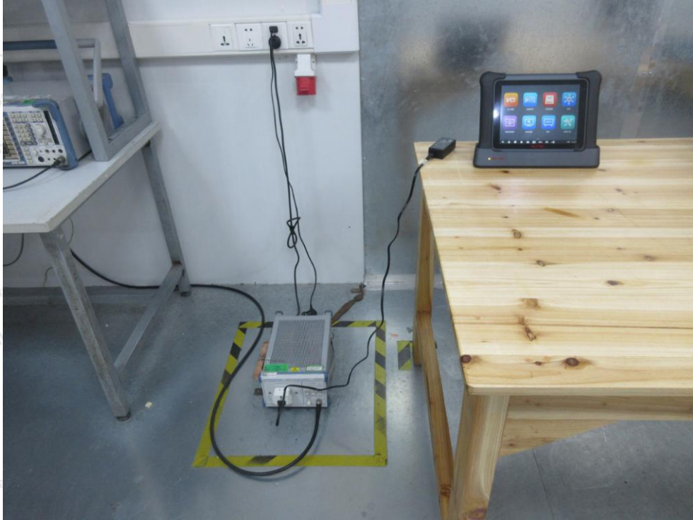
Photo of Power Line Conducted Emission Test
