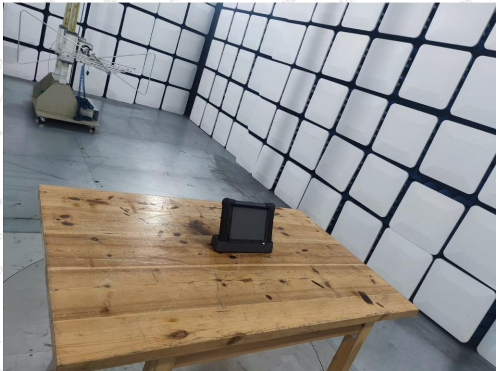
Photo of Radiation Emission Test
