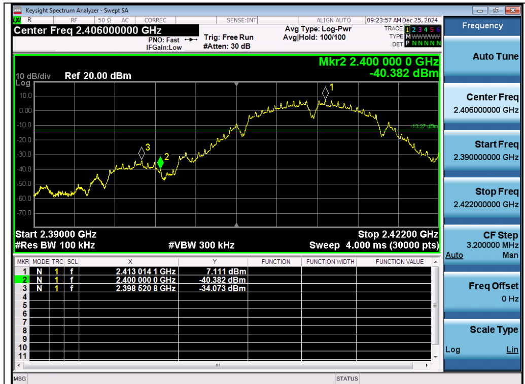
Test_Graph_802.11b_ANT1_2412_1Mbps_Lower Band Edge Emissions
