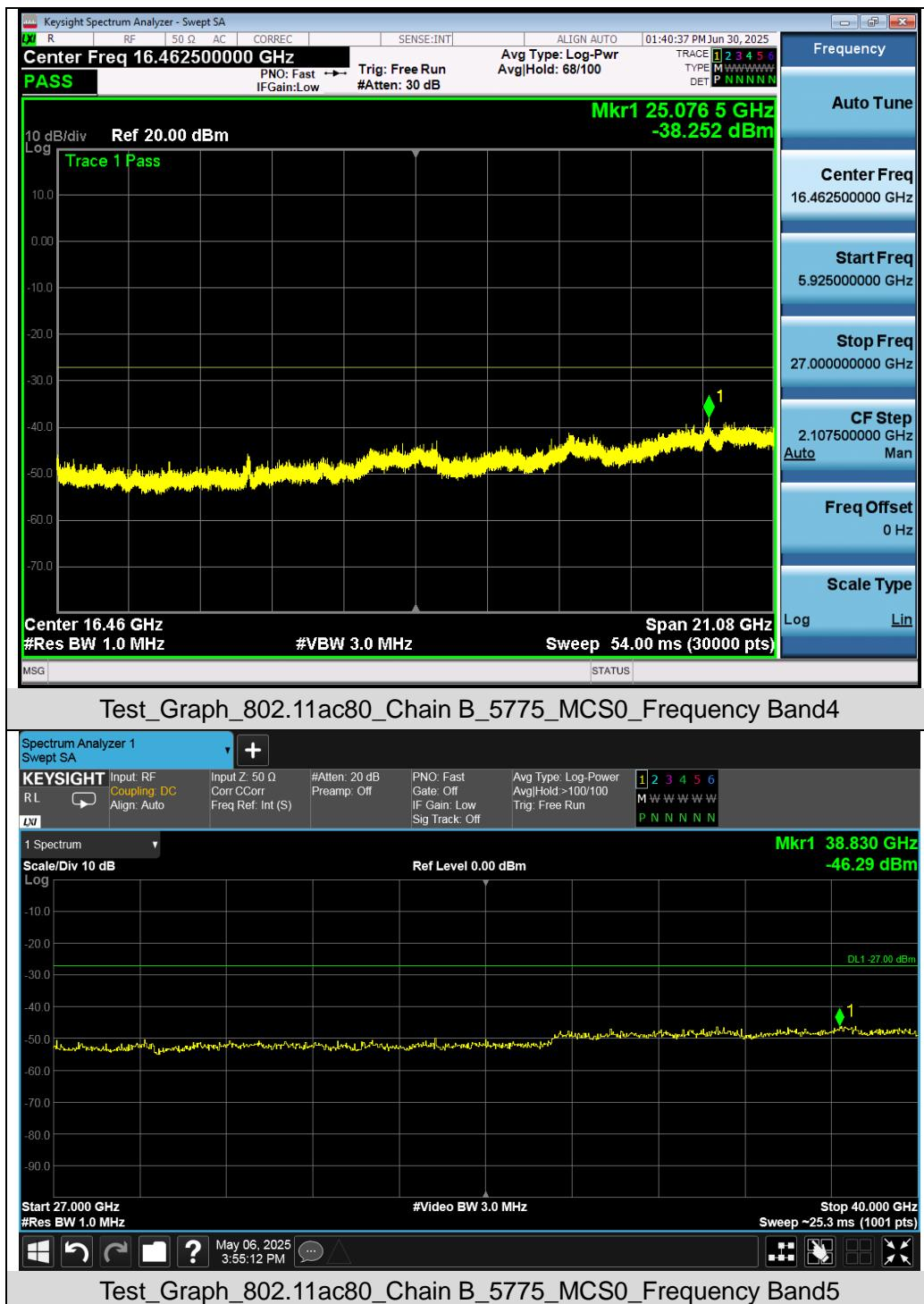
Note: The test data already includes the cable loss and antenna gain, and the margin of each chain is greater than 3.01dB. So MIMO data do not need to reflect.
