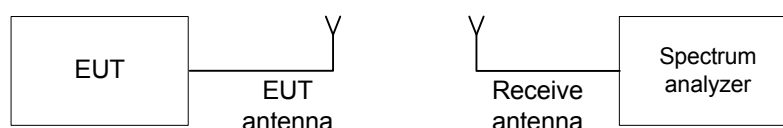
Figure 7.1.1 The 6 dB bandwidth test setup
