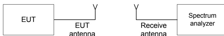
Figure 7.1.1 The 20 dB bandwidth test setup
