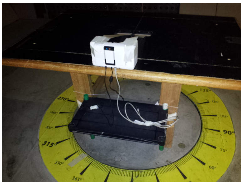
Photograph 8.2.2 Setup for radiated emission measurements, EUT cabling
