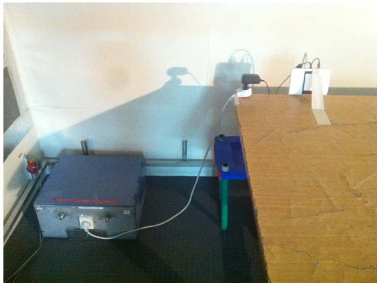
Photograph 8.1.1 Setup for conducted emission measurements
