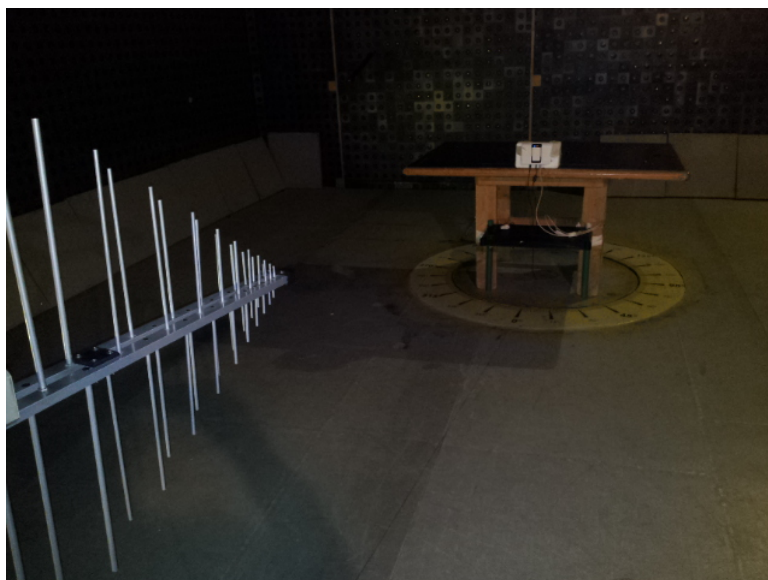
Photograph 8.2.2 Setup for radiated emission measurements, EUT cabling
