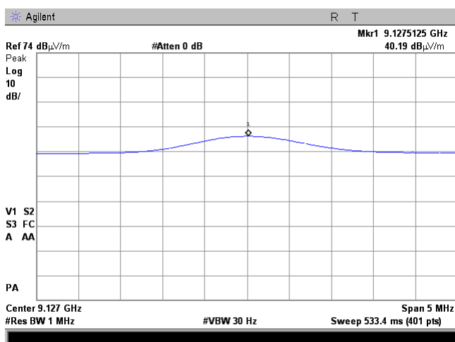
Plot 7.6.40 Radiated emission measurements at the tenth harmonic of mid carrier frequency
