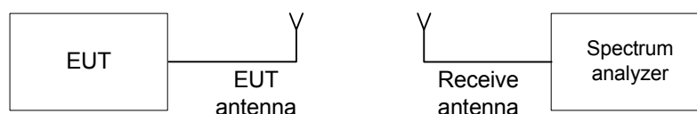
Figure 7.7.1 Band edge emission test setup
