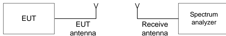
Figure 7.1.1 The 20 dB bandwidth test setup
