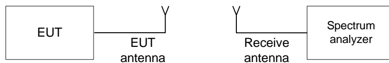
Figure 7.2.1 Carrier frequency separation test setup
