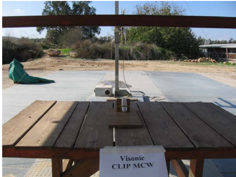
Figure 2 Radiated Emission Test Setup
