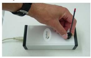
2. When inserting antenna take care to insert the bullet point connector into the connection terminal, as shown below.
