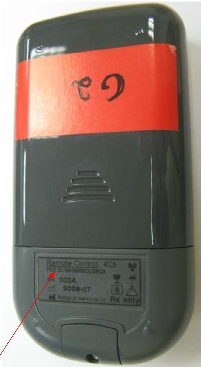
The label is located at the rear side panel of the Remote Control unit.
