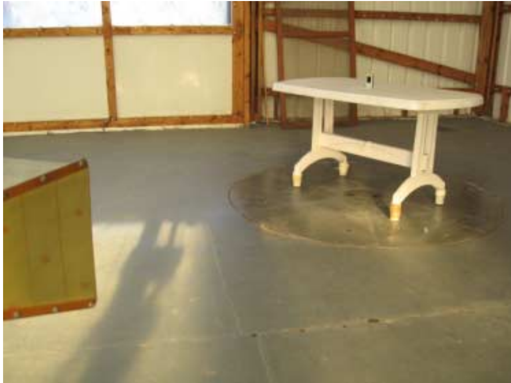
Photograph No.1 Setup for fundamental and spurious emission field strength measurements at OATS, EUT in vertical position (X-axis)
