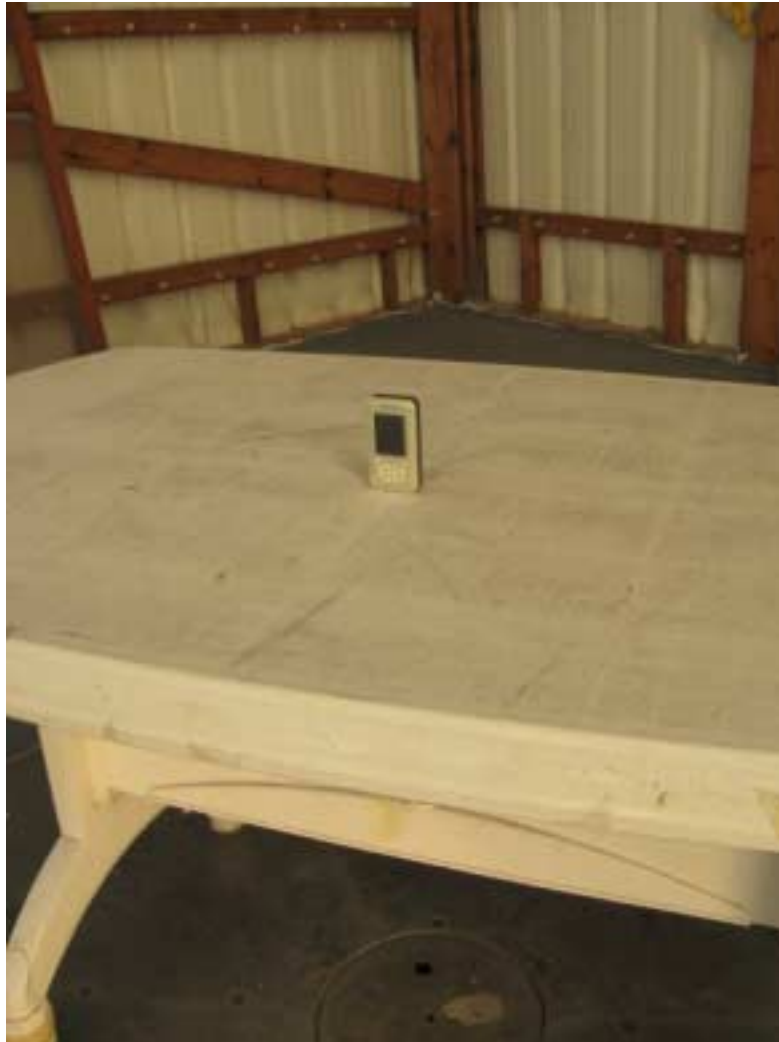
Photograph No.2 Setup for fundamental and spurious emission measurements at OATS, EUT close view in X-axis position
