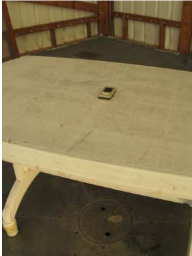
Photograph No.3 Setup for fundamental emission measurements at OATS, EUT close view in Y-axis position
