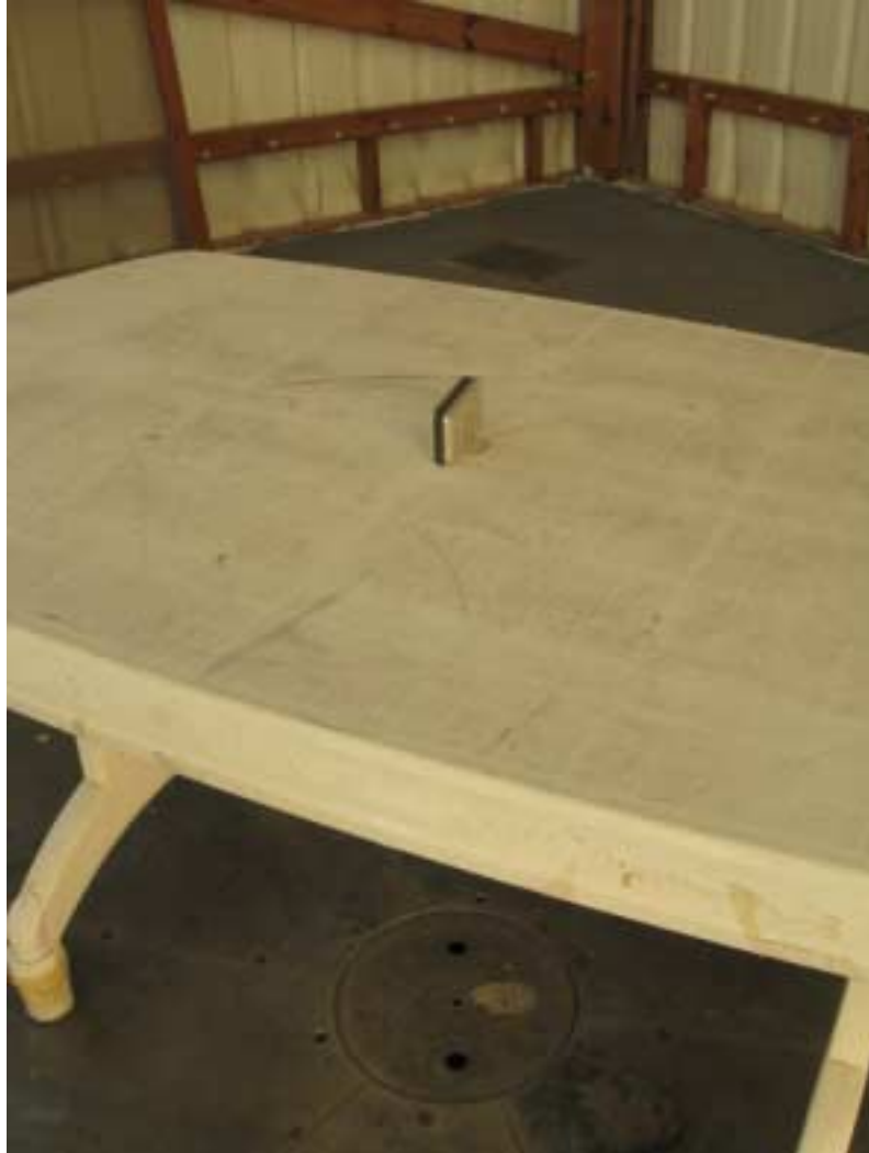
Photograph No.4 Setup for fundamental emission measurements at OATS, EUT close view in Z-axis position
