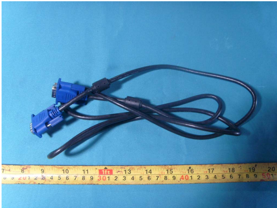
VGA Cable View
