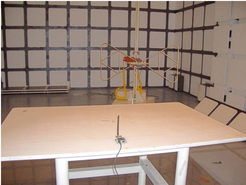
Radiation Emission Test Setup:
